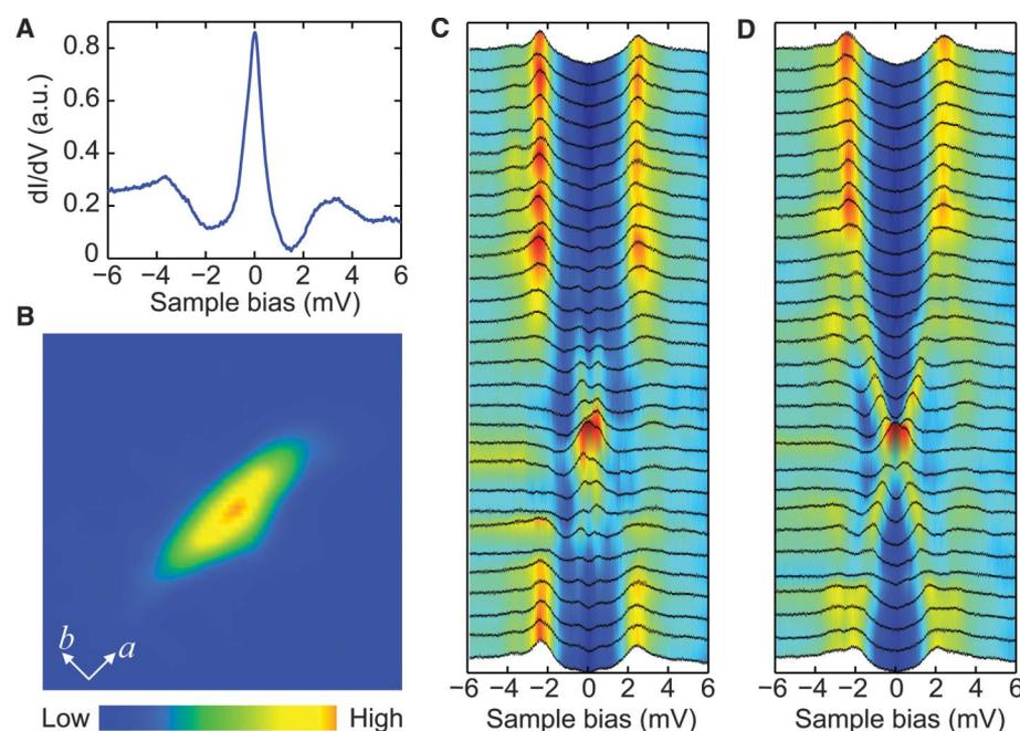
**Fig. 2.** The vortex core states. (A) STS (setpoint, 10 mV, 0.1 nA) on the center of a vortex core. (B) Zero-bias conductance map (40 × 40 nm<sup>2</sup>; setpoint, 10 mV, 0.1 nA) for a single vortex at 0.4 K and 1 T magnetic field. (C and D) Tunneling conductance curves measured at equally spaced (2 nm) distances along  $a$  and  $b$  axes.
